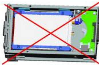
Wrong Installation (Hard disk is upward.)
